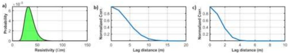
Figure 17: a) Log-Gaussian prior distribution for the field data inversion. b), and c) the spatial correlation functions associated with the assumed 2-D variogram model for the horizontal and vertical directions, respectively.
