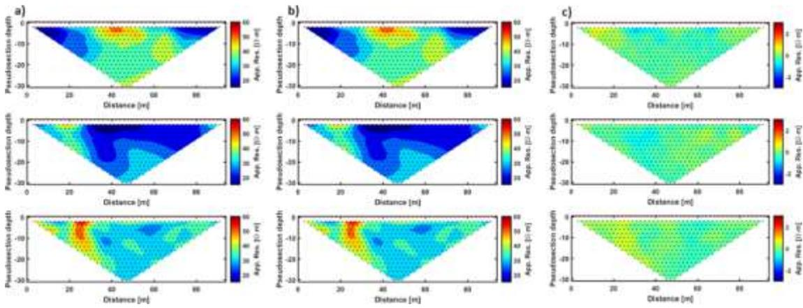
Figure 18: Some comparisons between (a) the network responses and (b) the desired output extracted from the validation set. In c) we represent the sample by sample difference between a) and b). Note the different color scale in c) with respect to a) and b).
