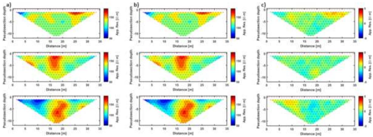
Figure 8: Some comparisons between (a) the network responses and (b) the desired (i.e., FE) output from the validation set. In c) we represent the sample by sample difference between a) and b). Note the different color scale in c) with respect to a) and b).
