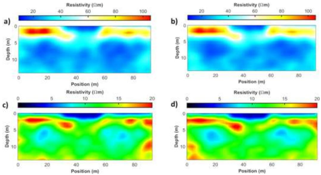
Figure 20: a) and b) the most likely solutions provided by the ES-MDA inversions when the ResNet and FE forward operator are employed, respectively. c) and d) Posterior standard deviations associated with the models shown in a) and b), respectively.
