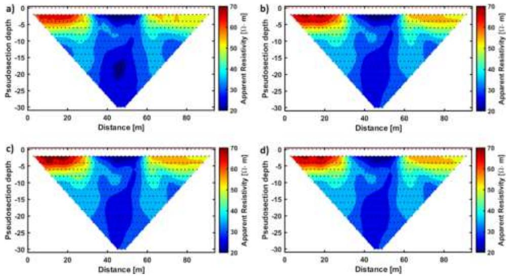
Figure 21: a) Observed data. b) Apparent resistivity pseudosection computed on the model shown in Figure 20a when the ResNet forward operator is used. c) Apparent resistivity pseudosection computed on the model shown in Figure 20a when the FE forward operator is used. d) Predicted data computed on the most likely model of Figure 20b with the FE code.
