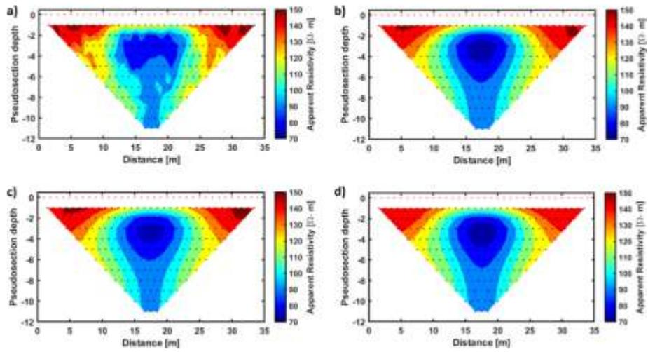
Figure 16: a) Observed data. b) Apparent resistivity pseudosection computed on the models shown in Figure 12a when the ResNet forward operator is used. c) Apparent resistivity pseudosection computed on the models shown in Figure 12a when the FE forward operator is used. d) Predicted data computed on the most likely model of Figure 12b with the FE code.
