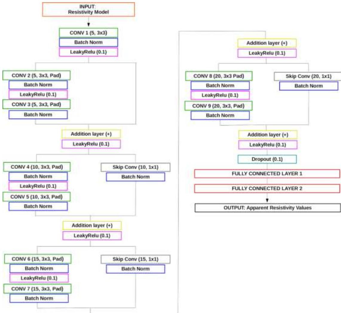
Figure 2: Representation of the employed ResNet architecture annotated with key parameters. For example, in the second convolutional layer “CONV 2” the term within bracket (5, 3x3, Pad) indicates that we employ 5 convolutional filters with size 3x3 and that zero-padding is applied. The only difference in the synthetic and field data applications concerns the dimension of input and output response. See the text for details.
