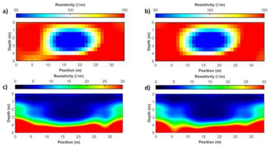
Figure 12: a) and b) the most likely models predicted by the DEMC inversions when the ResNet and FE forward operator are employed, respectively. c) and d) Posterior standard deviations associated with the solution shown in a) and b), respectively.
