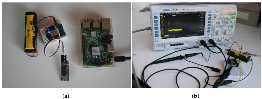
Figure 4. (a) The two prototype components: an edge unit (left) and the checkpoint storage server (right); (b) current measurement on the edge unit. The channel 1 of the oscilloscope measures the voltage on a 1 Ohm shunt resistor in series with the MCU. Channel 2 visualizes marker signals injected in the code.
