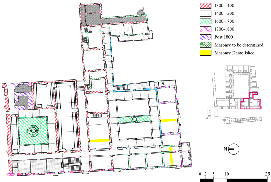
Fig. 5 First plan of a portion of the Certosa with the indication of the macro-constructive phases according to the legend
