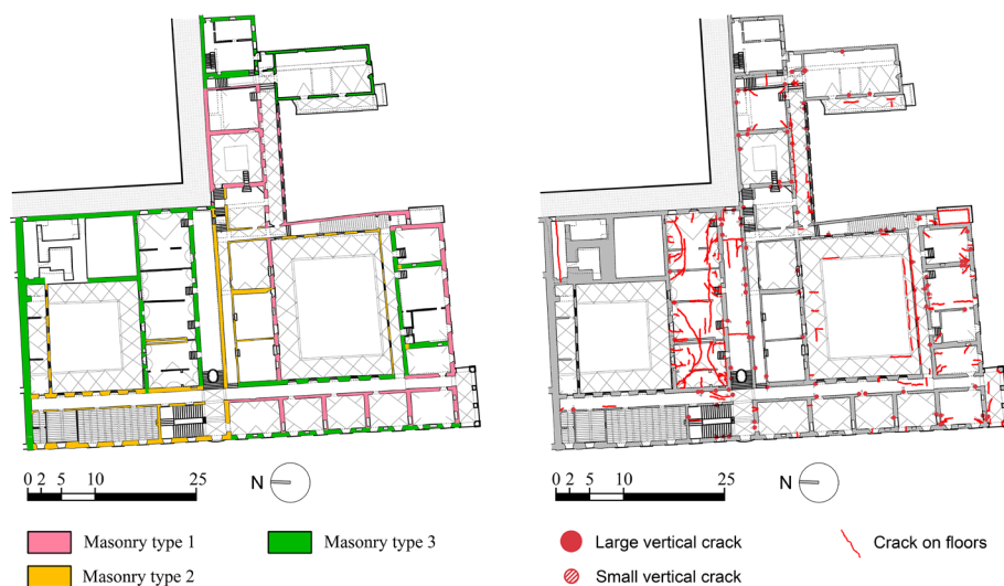
Fig. 7 Second plan of the portion of the monumental complex more in-depth analysed representing: a the survey of the masonry typologies, b the crack pattern survey
