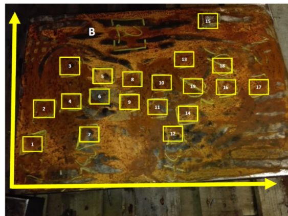
Figure 2. Sheet B, 410 × 620 × 90 (mm). The extraction positions of the test articles are highlighted in yellow.
