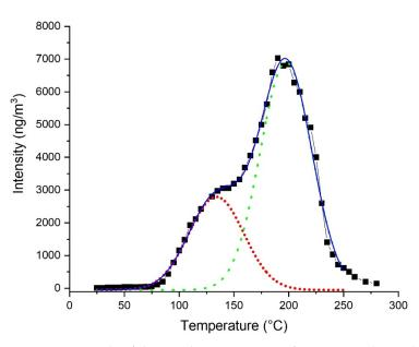
**Figure 4.** Example of thermo-desorption curve for PZ1-A soil sample (black squares). Deconvolution (blue line) indicates the occurrence of peaks centered at  $133 \pm 2$  °C (red dot, peak #1) and  $197.4 \pm 0.9$  °C (green short dash, peak #2). R-square = 0.99.
