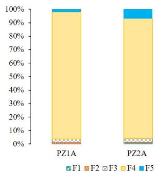
**Figure 3.** Normalized Hg F-fraction (wt%) extracted by each extractant solution for soil samples PZ1A and PZ2-A (F1 = distilled water, F2 = 0.01 M HCl + 0.1 M CH<sub>3</sub>COOH, F3 = 1 M KOH, F4 = 12 M HNO<sub>3</sub>, F5 = aqua regia).
