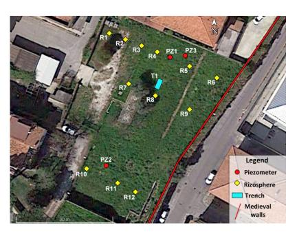
Figure 2. Sampling stations (PZ: boreholes/piezometers; T: trench; R: rhizosphere).
