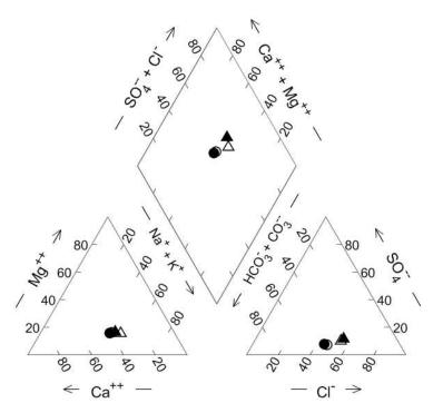
**Figure 6.** Piper diagram for the studied groundwater samples. Symbols: circle, PZ1; triangle: PZ2. Open and filled symbols refer to July 2019 (W1) and January 2020 (W2) samplings, respectively.
