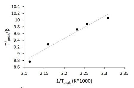
**Figure 5.**  $T^2_{peak}/\beta$  vs.  $1/T_{peak}$  (T in K) diagram. The slope of the linear fitting (dotted line) gives the activation energy ( $E_a/R$ ). R-square = 0.96.
