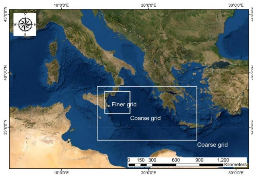
Fig. 5 - Coarse grids for Hellenic and the South-eastern Sicily areas (80x80 m cell width) employed in Delft3D-Flow simulation and finer grid (4x4 m cell width) employed in XBeach modelling.
