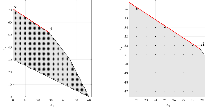
Fig. 5.2 An example in two dimensions with three objectives. The black points on the left figure are all the feasible solutions. All the nearest integer points parallel to the segment [\alpha, \beta] (there are many), are optimal for the first objective, while point (28, 52) is the unique lexicographic optimum for the given problem (i.e., considering the second objective too). The third objective plays no role in this case. On the right, a zoom around point \beta is provided, with some optimal solutions for the first objective highlighted (the ones with a bigger black spot).
