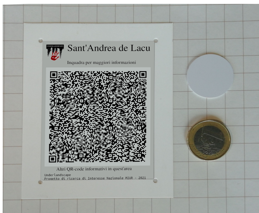
Figure 2. An NFC coin, a QR tag used in the prototype, and a 1 Euro coin for comparison on a paper with a square of 1 cm.
