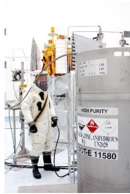
Figure 1 - Fuelling procedure requiring Hazmat suites for Messenger mission - credit NASA, public domain
