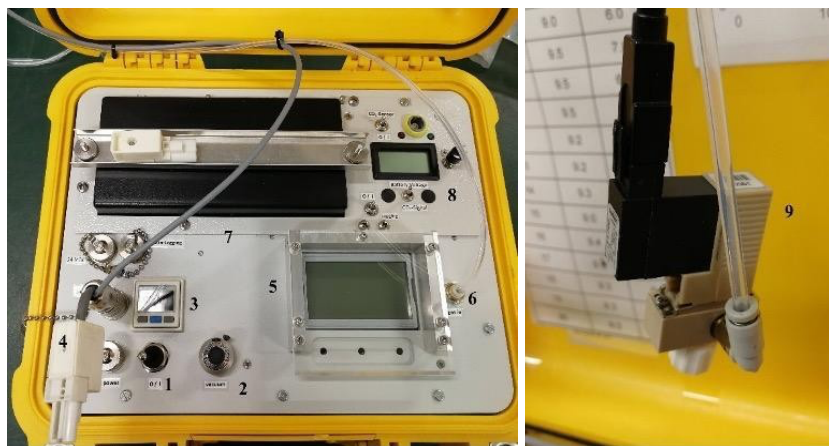
Figure 1. Sampling case used to transfer an accurate volume of breath sample in the SPE tube.
