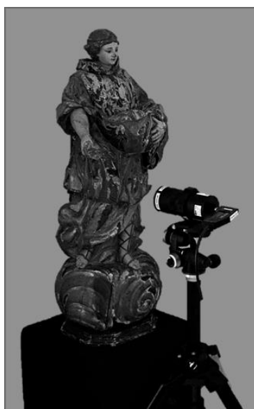
Figure 1. The use of a zoom lens for the in situ analysis of a polychrome sculpture
