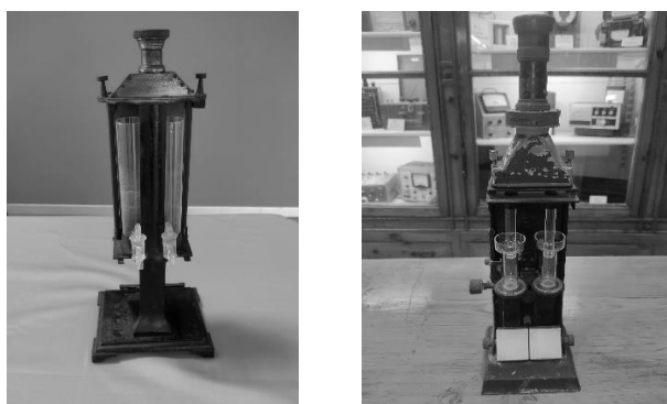
Figure 1. Two models of color comparator or visual colorimeter, from left to right, a Wolff's colorimeter (University of Pisa) and a Duboscq's colorimeter (University "La Sapienza" of Rome).
