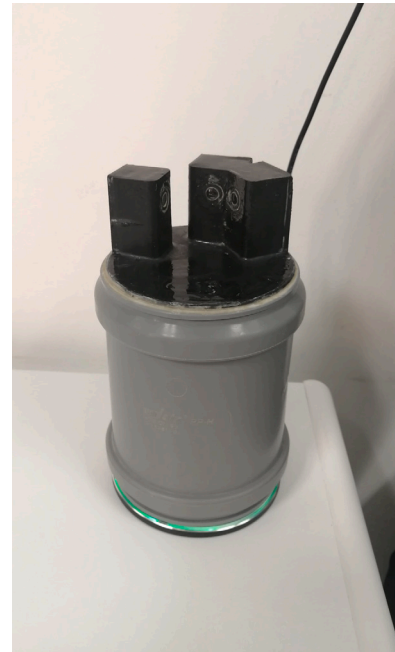
(b) The mobile version of the turbidimeter placed onto its wireless recharge station (the round base with a green light). The turbidimeter is ~17 cm high, with a diameter of ~10 cm. The cable is a standard USB-C cable that provides power to the charging station.
