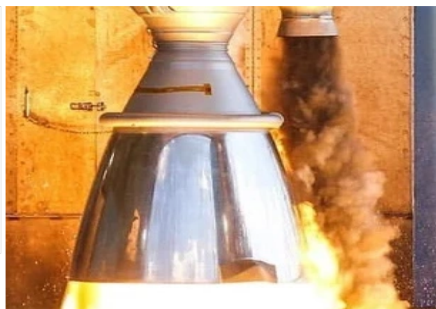
Figure 2: SpaceX's Merlin engine. On the right side of the thruster it is visible the exhaust from the gas generator fuel-rich combustion. Image Credit: Business Insider
