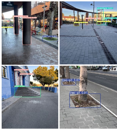
Fig. 17 YOLOv8 object detection model predictions. The image showcases the model's accurate identification and classification of various objects and corresponding probabilities in a collage of photos
