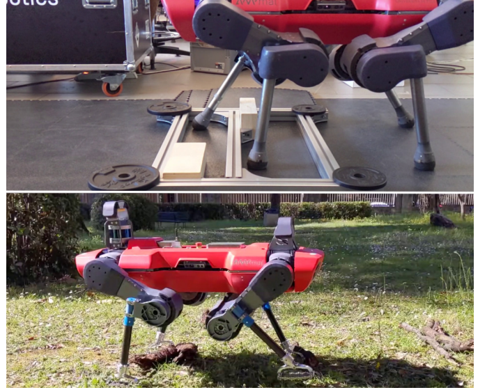
Fig. 1. ANYmal robot walking on rough terrain employing the proposed foothold planning algorithm based on a Convolutional Neural Network. The method searches for contact points that ensure a high contact surface and a high grip depending on the shape of employed feet.
