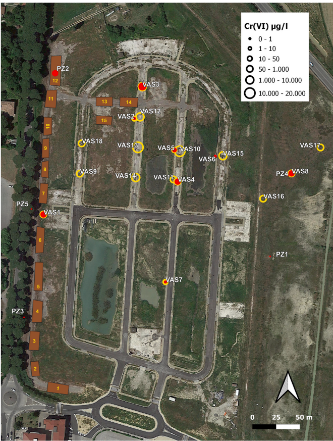
Fig. 6. Hexavalent chromium distribution in surface water from the drainage system during the dry (filled circles) and wet (open circles) seasons. The Cr(VI) concentration scale is shown.
