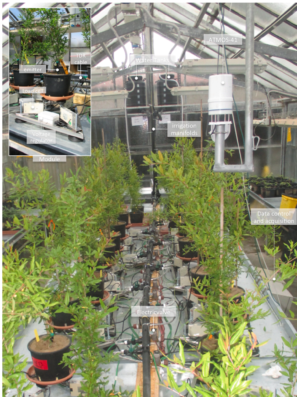
Fig. 1. Panoramic image of the HTS system. In detail, the main parts of a single module are shown.
