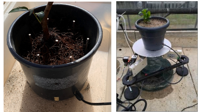
Fig. 3. TDR probes integrated into the pot (left) and the complete module (right) of the HTS system.
