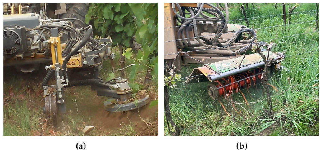
Figure 2. Tools employed in the two cutting-based strategies: the horizontal disc with axial cutting blades (a) and the wire-equipped mulcher (b).
