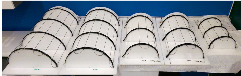
Figure 57. Finished Layer 4, 5 and 6 (from right to left) pipes on their storing and shipping masks.
