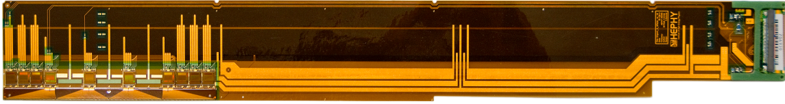
Figure 16. Fully loaded Origami_CE flexible PCB with dimensions 450.71 \times 57.39 \text{ mm}^2 . The 6 P-side and 4 N-side APV25 are located on the far left of the circuit.
