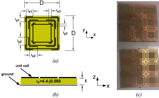
**Fig. 2.** (a) Unit cell geometry of the periodic surface-based chipless RFID, (b) side view of the proposed chipless tag, (c) chipless RFID prototypes.
