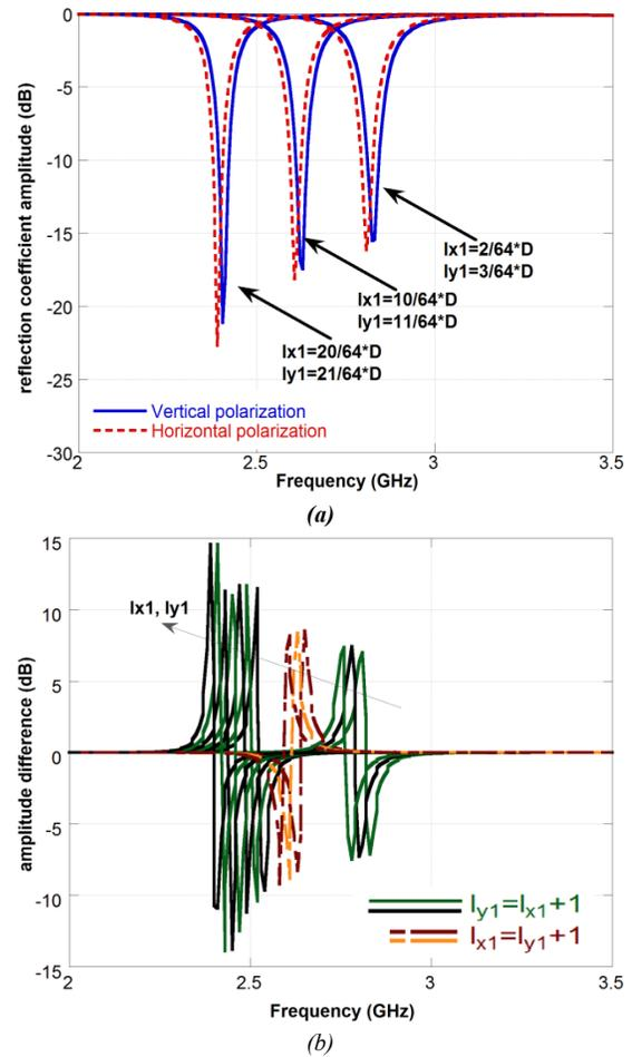
**Fig. 3.** (a) Amplitude of reflection coefficient for vertical and horizontal polarizations of an infinite array of 3-loop with stubs. (b) Amplitude difference between the reflection coefficients. The curves are obtained by progressively varying the length of the  $x$  and  $y$  directed stubs of the first loop and imposing  $l_{yj} = l_{xj} + 1$  or  $l_{xj} = l_{yj} + 1$ . The other stubs are fixed as:  $l_{x2} = l_{x3} = 2/64 D$ ,  $l_{y2} = l_{y3} = 4/64 D$ .
