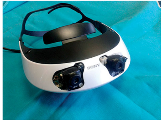
Figure 1. Wearable video see-through display. The head mounted stereoscopic video see-through display.
