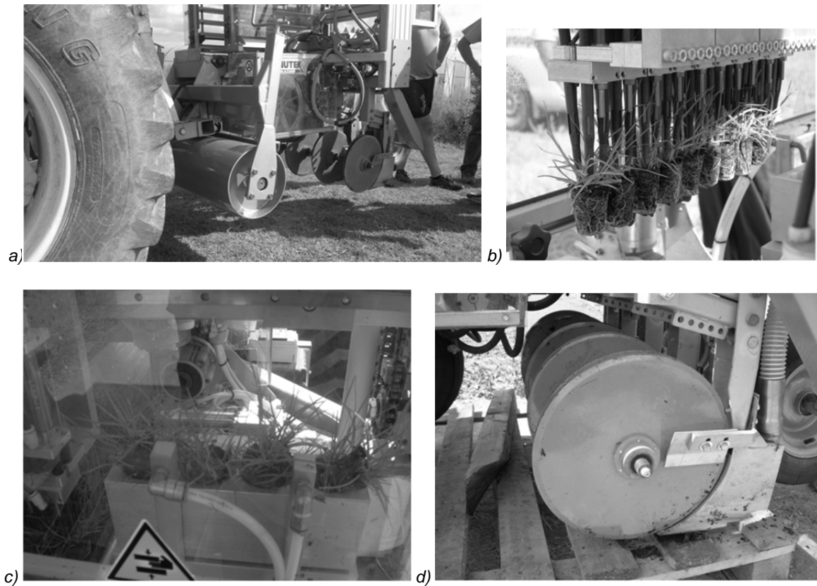
Figure 3: Automatic machine for warm season turfgrasses transplanting: a) machine view and detail of the front roll; b) claws for plant pick up; c) sliding chassis to deliver plants to furrowers; d) furrowers.
